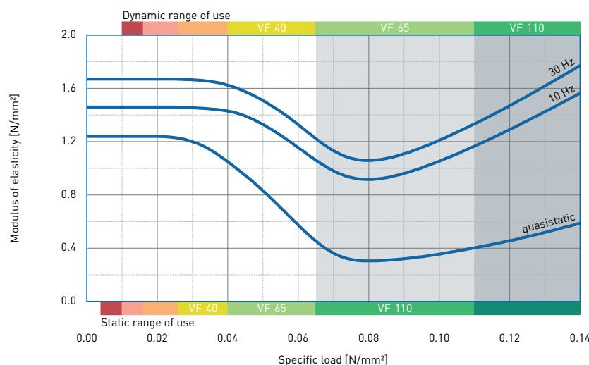
Dynamic test: sinusoidal excitation with an oscillating range of  $\pm 0.22$  mm at 10 Hz and  $\pm 0.08$  mm at 30 Hz
